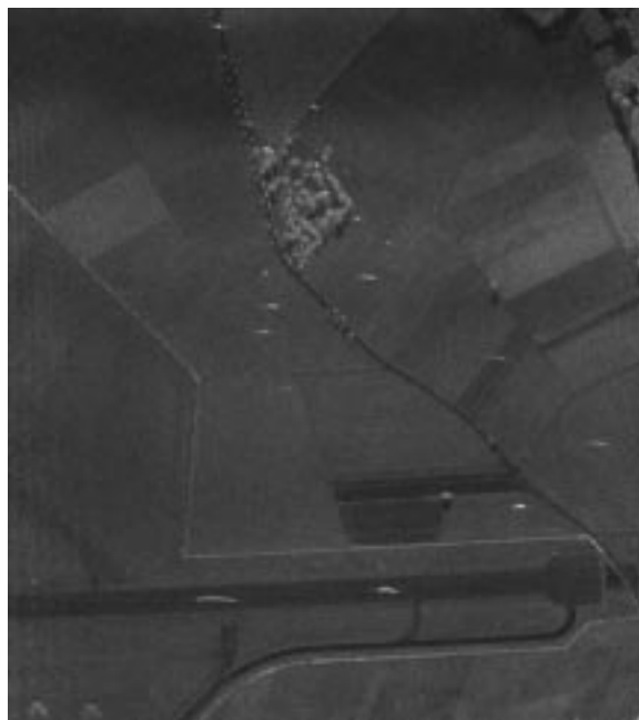
Figure 4. Multilook image generated from the same data as in Fig. 2, using a conventional SAR processor; the moving objects appear blurred and shifted or are even disappeared
