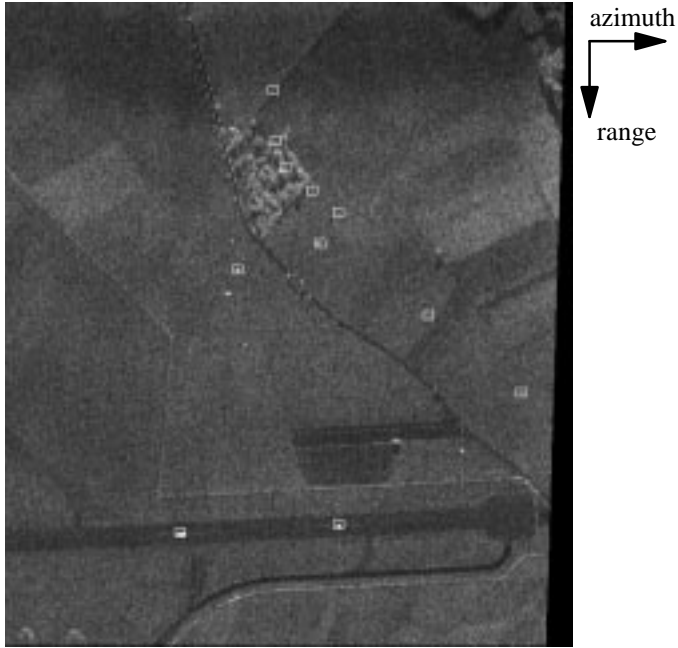
Figure 2. Single-look image from a sequence generated from simulated raw data of 15 moving objects superimposed on real clutter data; Detected moving objects are marked;
