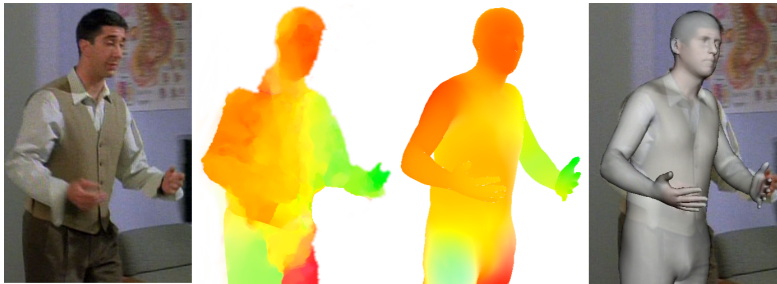
Fig. 1: Following our main idea we compute the optical flow between two consecutive frames and match it to an optical flow field estimated by our proposed optical flow renderer. From left to right: input frame, color-coded observed flow, estimated flow, resulting pose.
