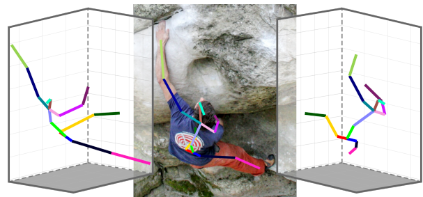
Figure 1. Our network predicts 3D human poses from noisy 2D joint detections. We use weakly supervised adversarial training without 2D to 3D point correspondences. Our critic networks enforces a plausible 3D pose while a reprojection layer projects the 3D pose back to 2D. Even strong deformations and unusual camera poses can be reconstructed.
