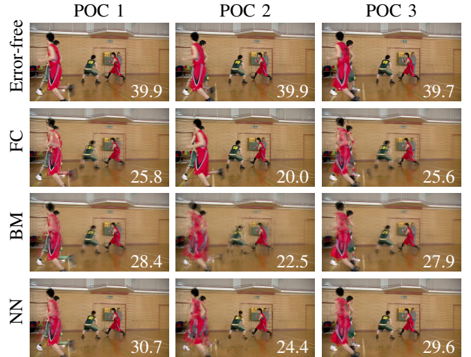
Fig. 6: The top row shows error-free decoded frames of the BasketballDrive sequence. In the other rows, POC 2 is estimated using NN, BM and FC approach. POC 1 and 3 are encoded with POC 2 in their reference picture lists. In each frame its corresponding \text{PSNR}_Y is given.
