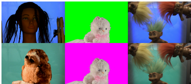
Figure 8: Evaluation dataset: (left) Composition of Castle and Dmitriy of Erofeev et al. 's [8] benchmark 5 in front of a realistic blue and green background respectively, (middle) composition of Alex (also [8]) in front of a pure and orthogonal green and purple background and (right) two consecutive frames with Trolls using our demonstrator.
