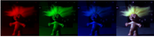
Figure 2: Images of a troll with yellow hair, that are captured with the same, static camera under varying monochromatic illuminations. It can be seen that the troll under green illumination appears detailed, while the red and blue illuminated images are blurry. This effect is called chromatic aberration, an effect caused by dispersion at the camera lens. The superposition of the three mono chromatic images is shown at the right. Here, the effect of chromatic aberration is visible as purple fringes.
