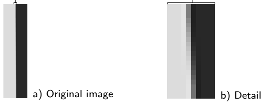
Fig. 4. Synthetic image used in the experiment. The edge is slightly slanted, so that feature points with a range of subpel coordinates can be detected.
