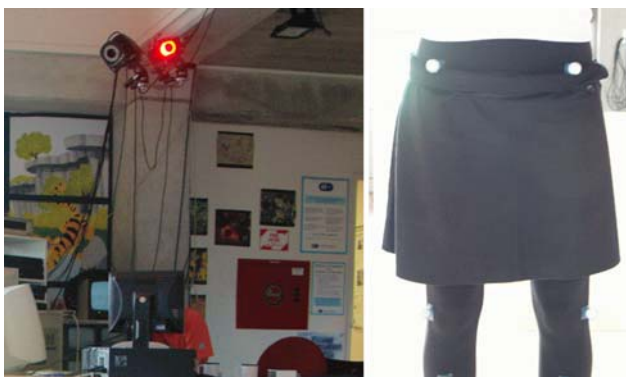
Fig. 17 The set-up for the quantitative error analysis. Left: The motion analysis system (and one of the strobe light cameras). Right: The subject with markers attached to the body
