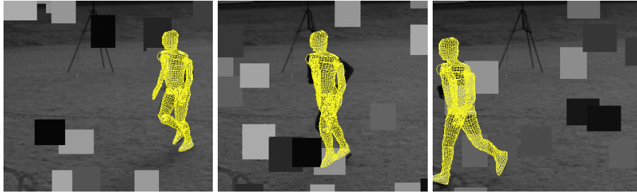
Fig. 7. Tracking of the jogging sequence with 20 occluding boxes and only samples from a walking motion being available for density estimation. The image contains few information on the arms. Hence, the arm pose is hallucinated from the walking prior. The legs, however, are tracked well, despite the unfitting prior.
