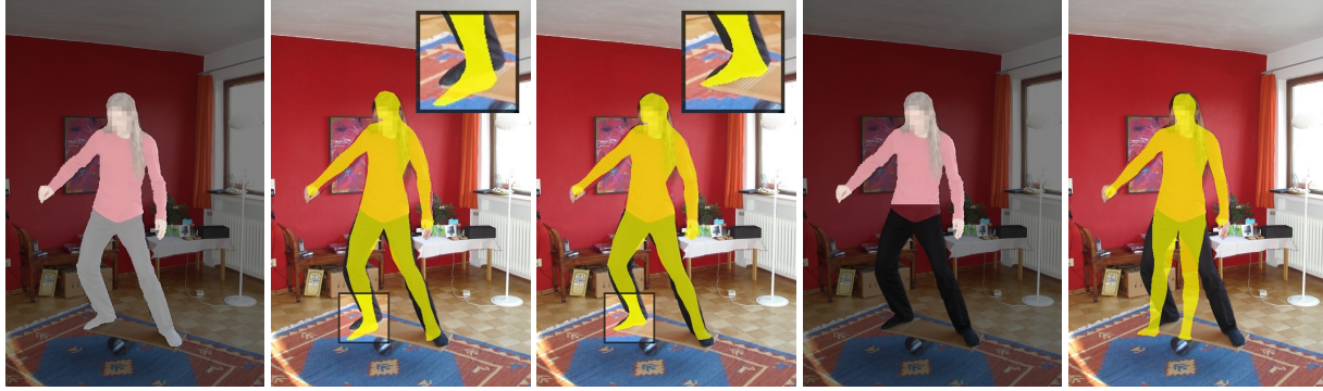
Figure 4. Leftmost three images: input silhouette, result with an orthographic (middle) and a projective camera (right). Rightmost two images: silhouette with simulated occlusion (from hips downwards) and estimation result.
