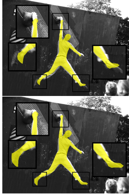
Figure 3. Estimation computed with an orthographic ( upper image ) and a projective camera ( lower image ).
