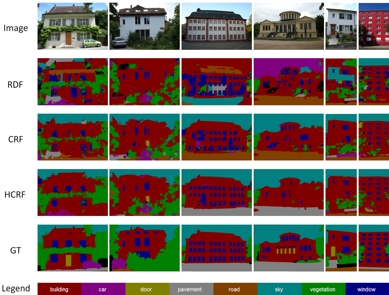
Figure 6. Qualitative classification results on testing images from the eTRIMS dataset. The hierarchical CRF model yields more accurate and cleaner results than the standard CRF and RDF. (1st-row) Testing images. (2nd-row to 5th-row) Classification results using the RDF classifier, the CRF model, the hierarchical CRF model (HCRF), and the ground truth (GT), respectively. (6th-row) Legend.
