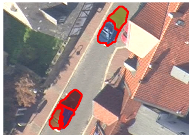
Figure 1. Example for a fully automatic moving object detection utilizing a superpixel segmentation.
