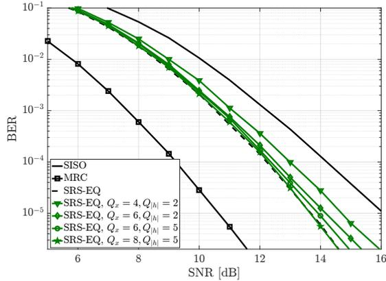
Fig. 4. The resulting BER comparison after SRS-EQ cooperation with  $\alpha_p = 15\%$ . SISO and MRC are benchmarked with  $\alpha_p = 0\%$  and  $\alpha_p = 100\%$  respectively. SRS-EQ is the ideal case of cooperation without quantizer, and for the non-ideal schemes, two quantizers are used,  $Q_x^{\text{EQ}}$  with  $Q_x$  bits resolution and  $Q_{|h|}^{\text{EQ}}$  with  $Q_{|h|}$  bits resolution.
