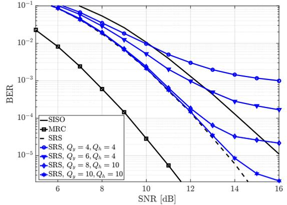
Fig. 3. The resulting BER comparison after SRS cooperation with  $\alpha_p = 15\%$ . SISO and MRC are benchmarked with  $\alpha_p = 0\%$  and  $\alpha_p = 100\%$  respectively. SRS is the ideal case of cooperation without quantizer, and for the non-ideal schemes, two quantizers are used,  $Q_h^{\text{SRS}}$  with  $Q_h$  bits resolution and  $Q_y^{\text{SRS}}$  with  $Q_y$  bits resolution.
