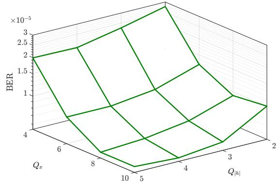
Fig. 5. BER for SRS-EQ depending on  $Q_x$  and  $Q_{|h|}$  for a fixed SNR = 14 dB.  $Q_x$  and  $Q_{|h|}$  give the resolution of  $Q_x^{\text{EQ}}$  and  $Q_{|h|}^{\text{EQ}}$  respectively.
