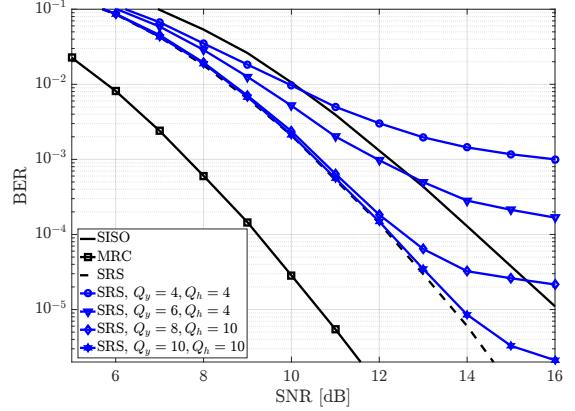
Fig. 3. The resulting BER comparison after SRS cooperation with  $\alpha_p = 15\%$ . SISO and MRC are benchmarked with  $\alpha_p = 0\%$  and  $\alpha_p = 100\%$  respectively. SRS is the ideal case of cooperation without quantizer, and for the non-ideal schemes, two quantizers are used,  $Q_h^{SRS}$  with  $Q_h$  bits resolution and  $Q_y^{SRS}$  with  $Q_y$  bits resolution.
