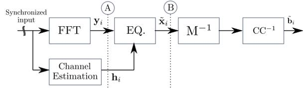
Fig. 2. Block diagram of a generic receiver  $Y_i \forall i$ , the input signal is assumed synchronized in  $t$  and  $f$  domain and with the cyclic prefix removed.
