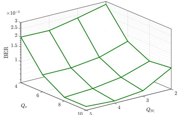
Fig. 5. BER for SRS-EQ depending on  $Q_x$  and  $Q_{|h|}$  for a fixed  $\text{SNR} = 14$  dB.  $Q_x$  and  $Q_{|h|}$  give the resolution of  $Q_x^{\text{EQ}}$  and  $Q_{|h|}^{\text{EQ}}$  respectively.
