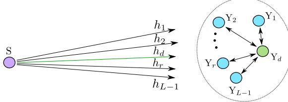
Fig. 1. System model, one source  $S$  and  $L$  receivers close to each other.  $S$  communicates a message to a destination node  $Y_d$ , all remaining receivers may serve as relays in order to assist  $Y_d$  in decoding the message. Independent channels  $h_d, h_1, \dots, h_{L-1}$  are assumed.
