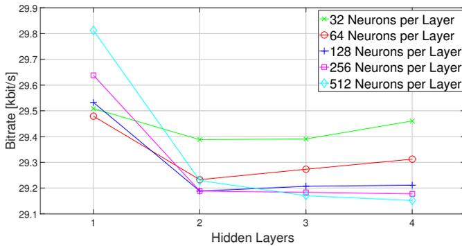
Fig. 6. Bitrate across number of neurons and layers of the artificial neural networks. Increasing the number of layers above two did not yield substantial benefits and the number of layers could be kept at two to reduce the computational complexity. A resolution of 6 bit/symbol was used to generate the depicted results.
