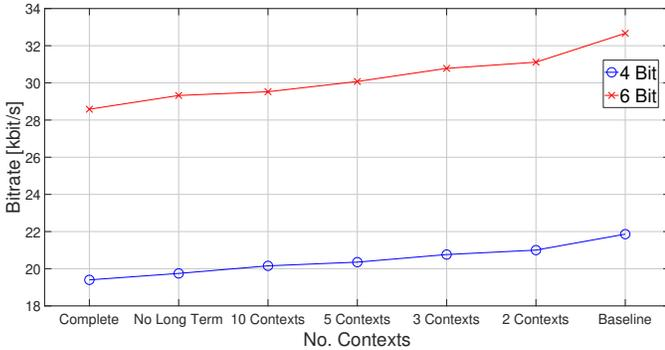
Fig. 5. Bitrate across the number of considered contexts per subband of the lossless codec. The single context was  $[0, -1]$ , i.e. the same subband but the previous time step, and served as reference to assess the benefit of context mixing. Invalid contexts like  $[-1, 0]$  in the first subband were ignored.
