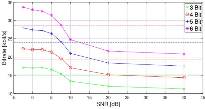
Fig. 4. Mean bitrate across signal-to-noise ratio (SNR) of the lossless codec on the test set. A considerable increase in bitrate with decreasing SNR was observed. The cause are more subbands that are selected at low SNRs. The dashed lines indicate the mean bitrate across the test set. These results were obtained using the complete set of contexts given in Table II.
