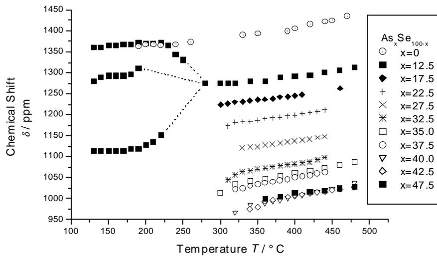
**Figure 2:** Dependence of  $^{77}\text{Se}$  chemical shift on Composition and Temperature in As-Se glasses.
