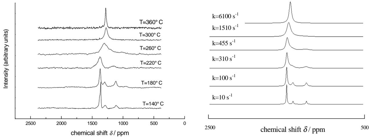
**Figure 5:** Temperature dependence of the  $^{77}\text{Se}$  NMR-spectra of As-Se melt containing 12.5 mole% As. Left: experimental spectra; right: simulations using a three-site exchange model (see text). In the simulation plots, the chemical exchange rates assigned to the respective temperatures are indicated.
