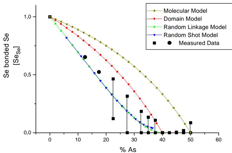
**Figure 10:** Comparison of the different scenarios with respect to the fraction  $f_1$  of the Se-only bonded Se atoms. Possible ranges of  $f_1$  deduced from the analysis of the experimental  $^{77}\text{Se}$  chemical shifts are indicated (see text).
