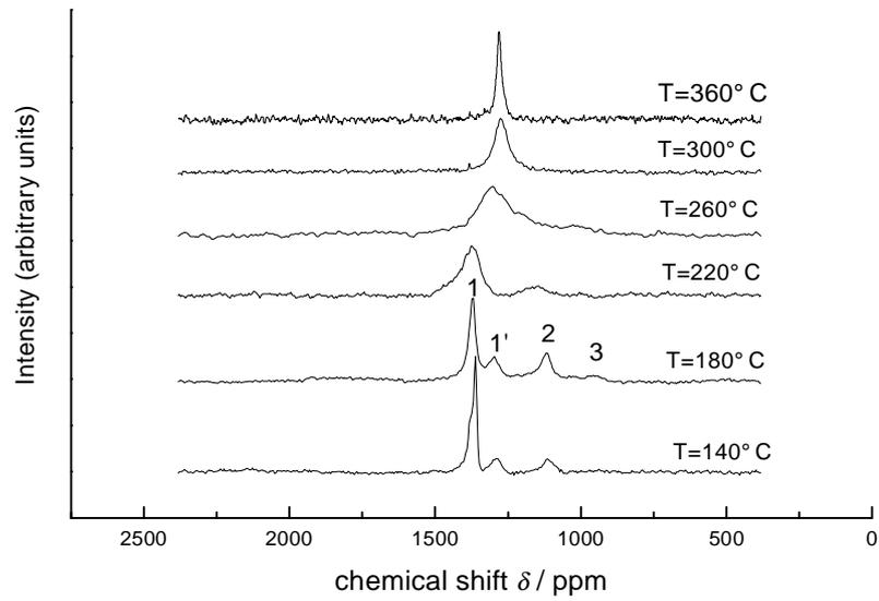
**Figure 1:** Experimental temperature dependent  $^{77}\text{Se}$  NMR spectra of  $\text{As}_{12.5}\text{Se}_{87.5}$  melt
