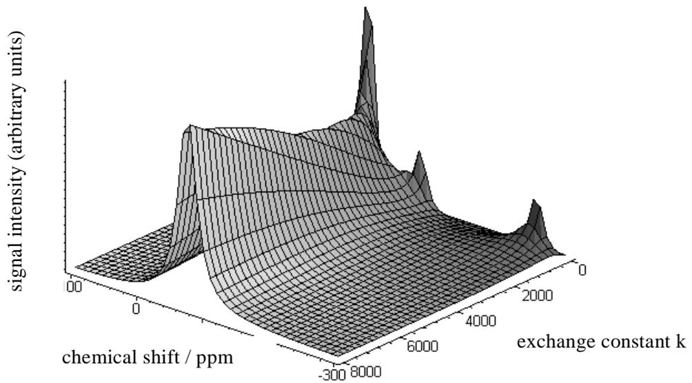
**Figure 4:** Chemical Exchange Simulation of  $^{77}\text{Se}$  NMR-Spectra: Lineshapes are shown as a function of exchange rate constant  $k$ . For further discussion, see text.
