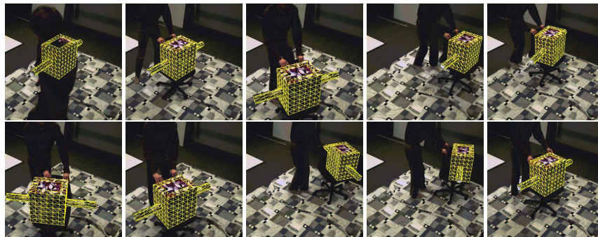
Fig. 8. Pose estimates for 10 of 570 frames. The sequence contains several difficulties for tracking: a rich textured and non-static background, shadows, occlusions, and other moving objects. Only one camera view is shown.
