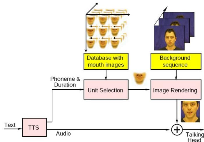
Fig. 2. The system architecture of the image-based talking head synthesizer
