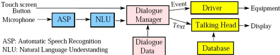
Fig. 5. Architecture of the human-car communication system.
