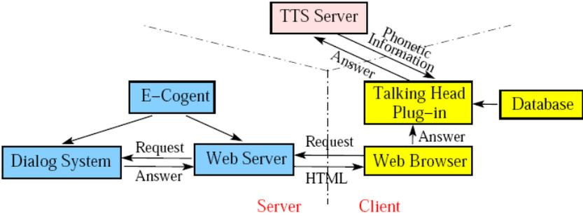
Fig. 3. Architecture of the E-Cogent application.
